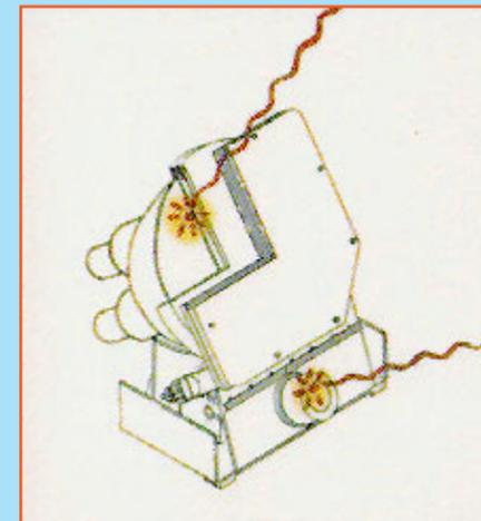
BATSE - the all-sky monitor for Compton is designed to detect gamma-ray bursts and search the sky for other transient emission.
