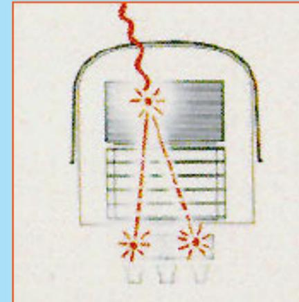
*EGRET is the highest energy experiment onboard Compton with sensitivity up to 30 GeV.*
