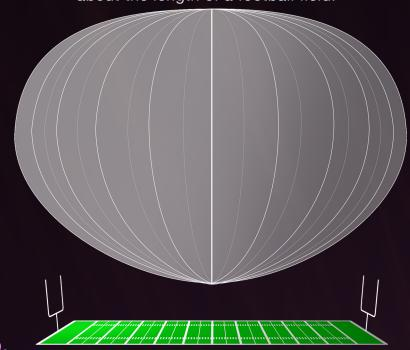
ComPair's maximum altitude is about 133,000 feet (40,000 meters). That's more than three times the cruising altitude of a commercial airplane.
