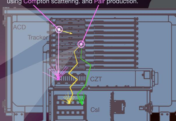
**COMPTON SCATTERING** A gamma ray hits an electron and transfers some of its energy to it, lowering its energy. The scattered electron, if tracked, can help scientists improve their knowledge of the original gamma
